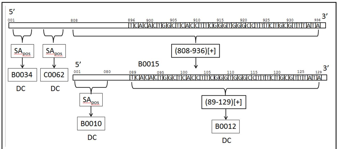
**Figure 8.** An expanded instance of BBa\_I0462, which demonstrates key features of SBOL:Core:model. In this instance, the BBa\_B0015 component of BBa\_I0462 from the examples above is composed of two elements itself, BBa\_B0010 and BBa\_B0012. The letters of the DNA sequence in the top *DnaComponent* is omitted, so only the sequence corresponding to BBa\_B0012 is shown.
